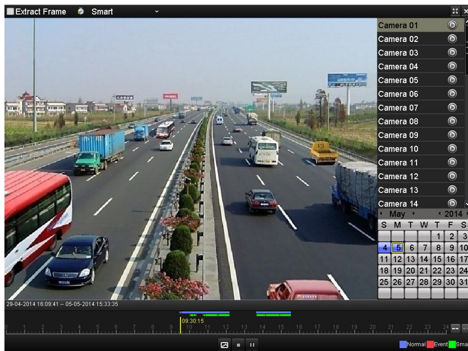
Figure 6.13 Smart Playback Interface
