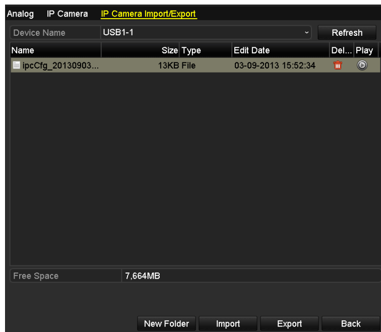
Figure 2. 14 Import IP Camera Configuration File
