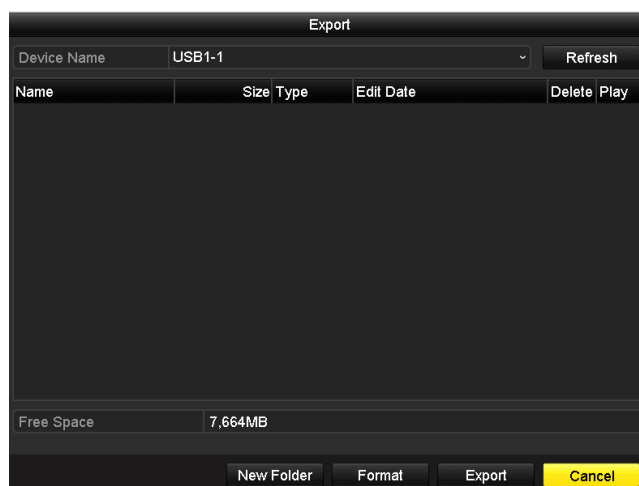
Figure 7.16 Export Video Clips Using USB Flash Drive
