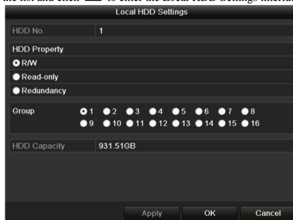
Figure 11.11 Local HDD Settings Interface
