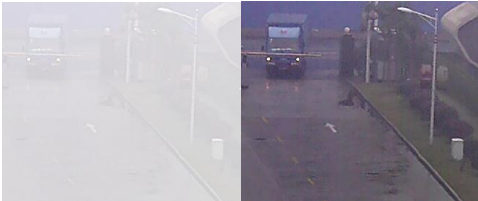
Figure 3. 5 A Comparison of the Details Before and After Defogging
