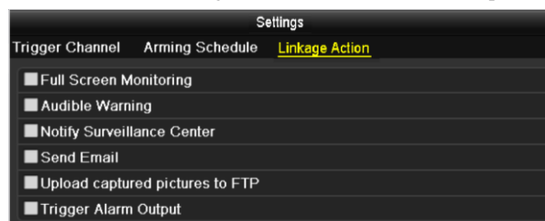
Figure 8. 4 Set Alarm Linkage Actions of Motion Detection
