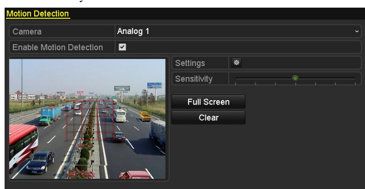
Figure 8.1 Set Detection Area and Sensitivity
