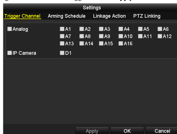
Figure 8.16 Set Trigger Camera of VCA Alarm
