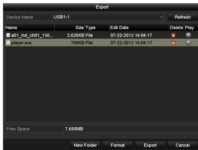
Figure 7.13 Checkup of Event Export Result Using USB Flash Drive
