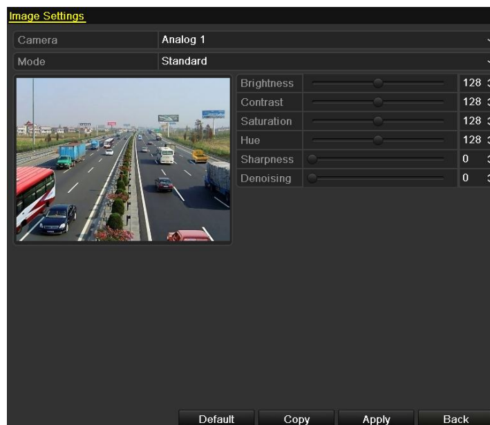
Figure 12. 4 Image Settings Interface for Analog Camera Connected to Other Series
