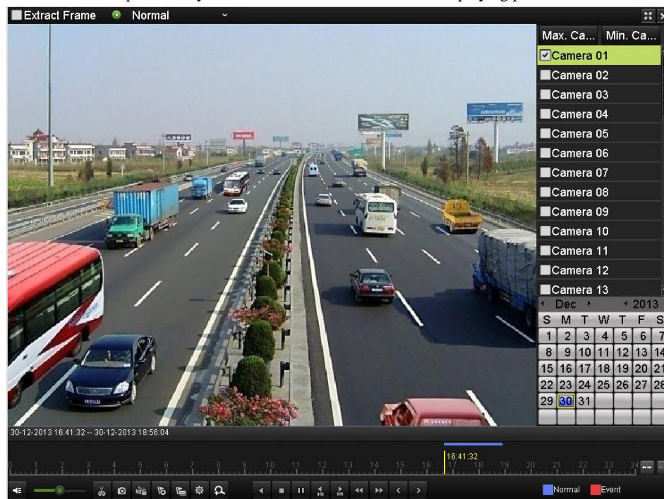
Figure 6.4 Interface of Playback by Time
