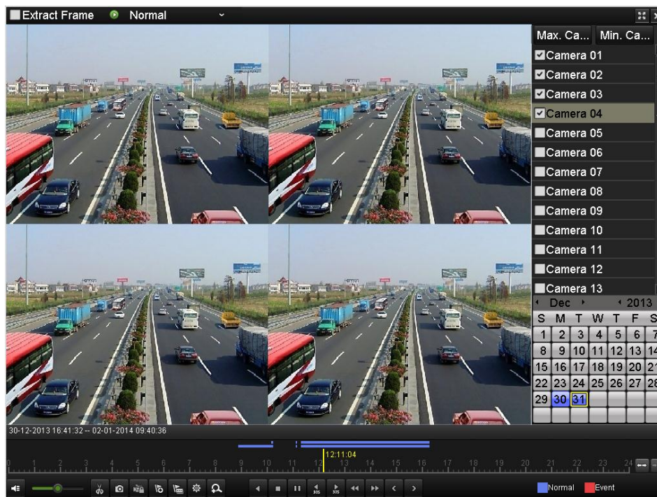
Figure 6. 20 4-ch Synchronous Playback Interface
